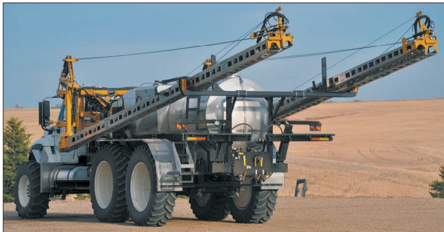
The Sprayflex sprayer with a 3,100 gallon tank and 150-foot boom transports in a tight package, respecting the fact that most producers who will use a machine of this size have land spread over large areas. | SPRAYFLEX PHOTO
