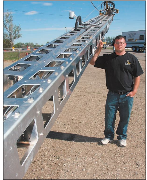
Jay Mercil says the design of the original Sprayflex aluminum boom allows him to extend the basic 100 foot boom up to 150 feet and wider.
