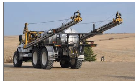
COMPACT FOLD: The 150-foot boom folds for transport.
